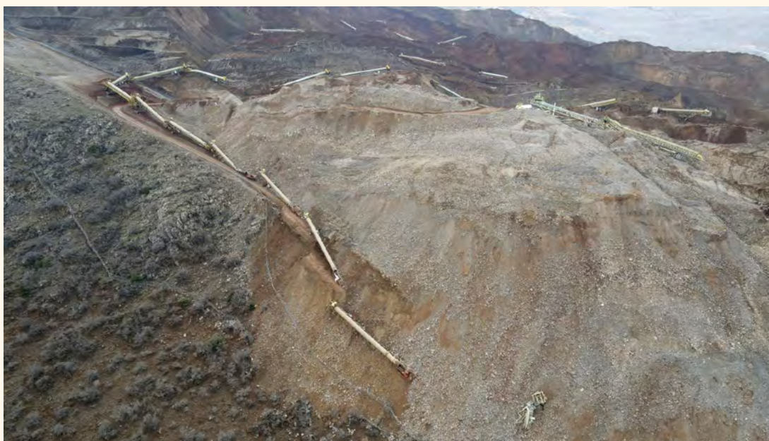
Image 8: The landslide at the Coper gold mine near Ilıc village, eastern Turkey. (Source: Bloomberg )
